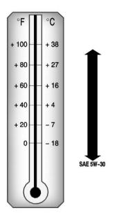
Cold Temperature Operation: In an area of extreme cold, where the temperature falls below −29°C (−20°F), an SAE 0W-30 oil should be used. An oil of this viscosity grade will provide easier cold starting for the engine at extremely low temperatures. When selecting an oil of the appropriate viscosity grade, be sure to always select an oil that meets the required specification, dexos™. See "Specification" for more information.
